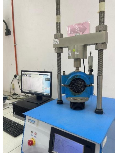
Figure 3. Marshall Stability Test
