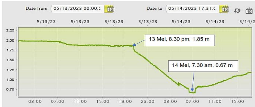
Figure 3. Equipment failure that causes the river level to drop
