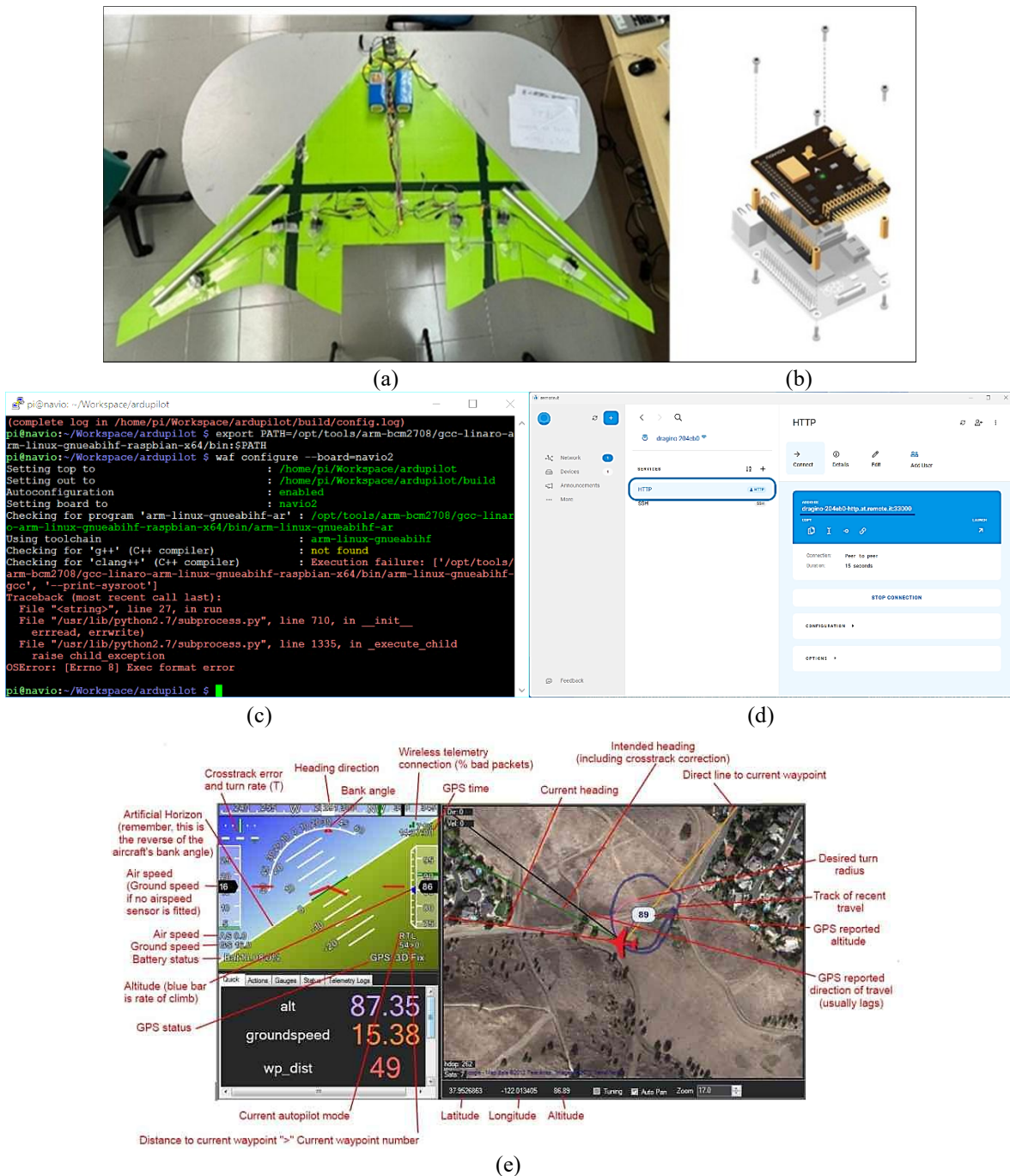
Figure 3. (a) the Iron Bird, (b) the Navio2 IMU/controller mounted on Raspberry Pi4 computer, (c) Navio2 programming interface, (d) Remote.it interface, and (e) Mission Planner GCS suite (ardupilot.org)
