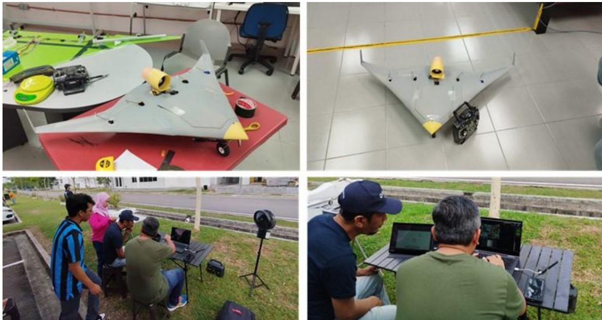
Figure 4. 1:2 scale POC model and navigation functionality test
