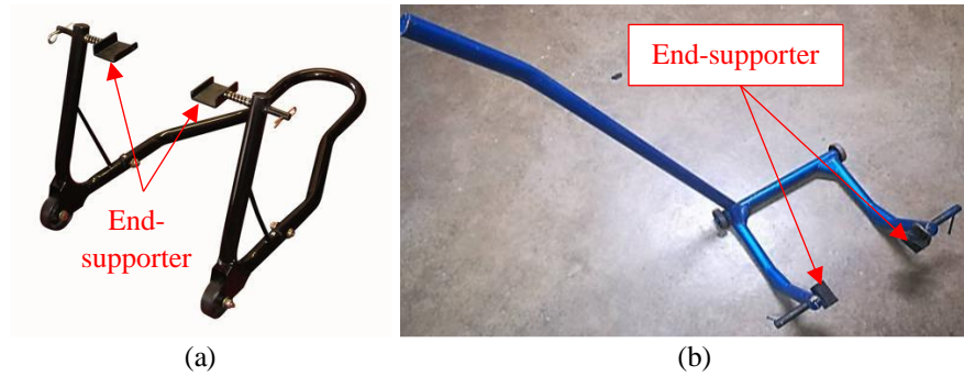
Figure 1. (a) Conventional paddock stand, and (b) RhiNO v1.0
