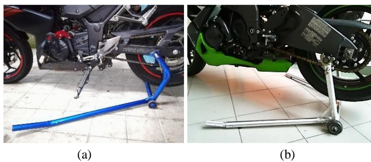
Figure 14. (a) RhiNO v1.0, and (b) RhiNO v2.0 in action
