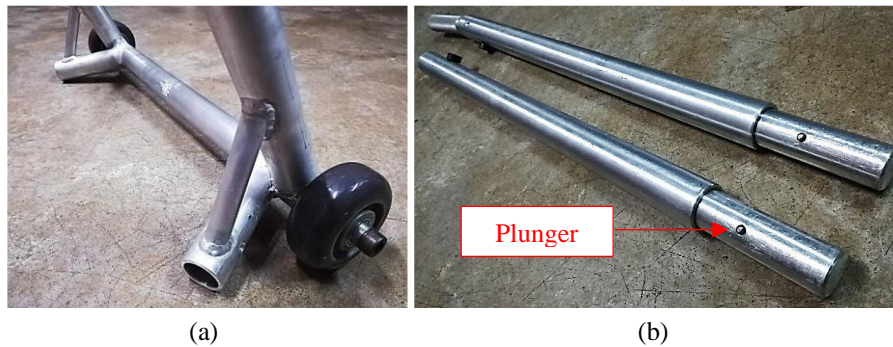
Figure 9. (a) Frame of the RhiNO v2.0 base after welding, and (b) Handle of the RhiNO v2.0 after press fitting
