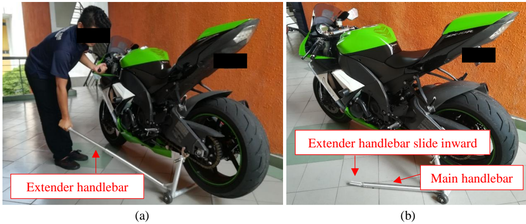
Figure 12. (a) Single user demonstration of RhiNO v2.0 and (b) The RhiNO paddock stand with superbike's rear tire lifted
