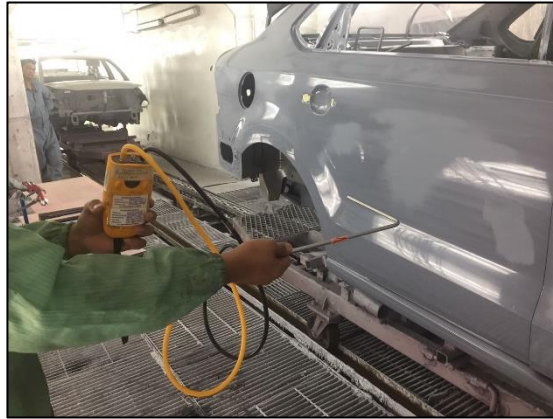
Figure 6. Air flow checking
