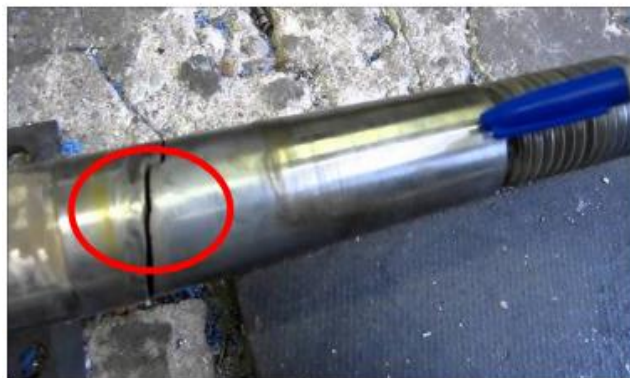
Figure 2. Example of transverse crack on solid shaft in Marine.
