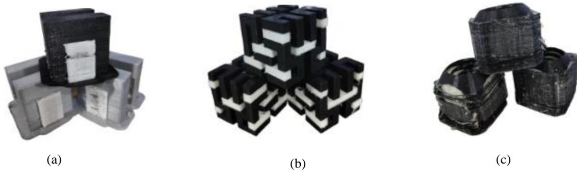
**Figure 8.** PLA sample with PVA support (a) Simple (b) Medium (c) Complex
