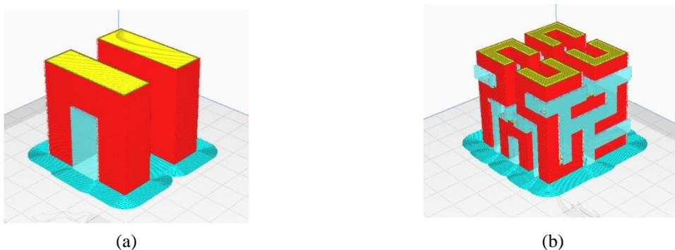
**Figure 3.** Support structure after slicing for (a) simple cube, and (b) Hilbert cube
