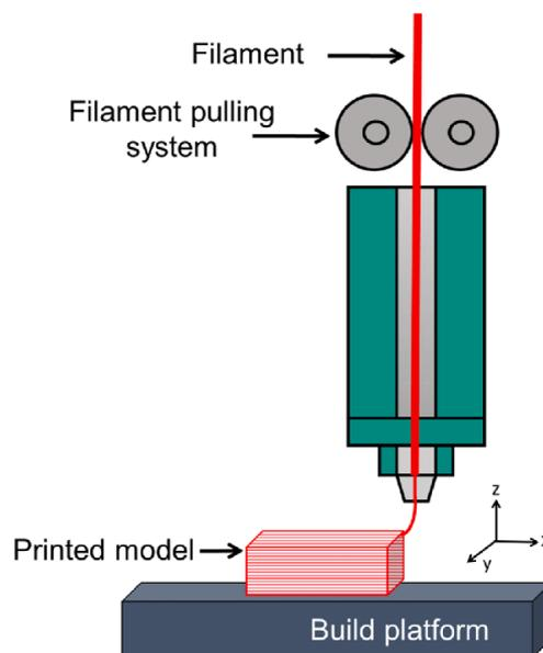
**Figure 1.** Schematic Diagram of FDM
