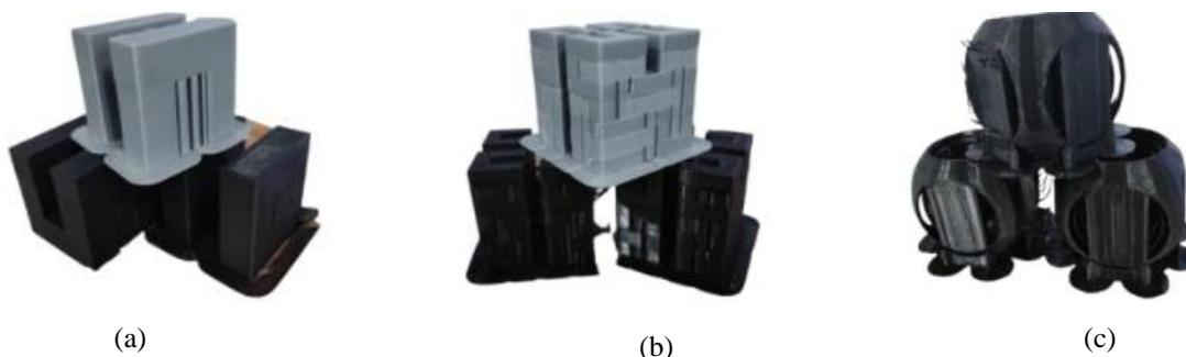
**Figure 7.** PLA samples with PLA support (a) Simple (b) Medium (c) Complex
