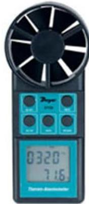
**Figure 2.** Thermo-anemometer used to conduct field measurements
