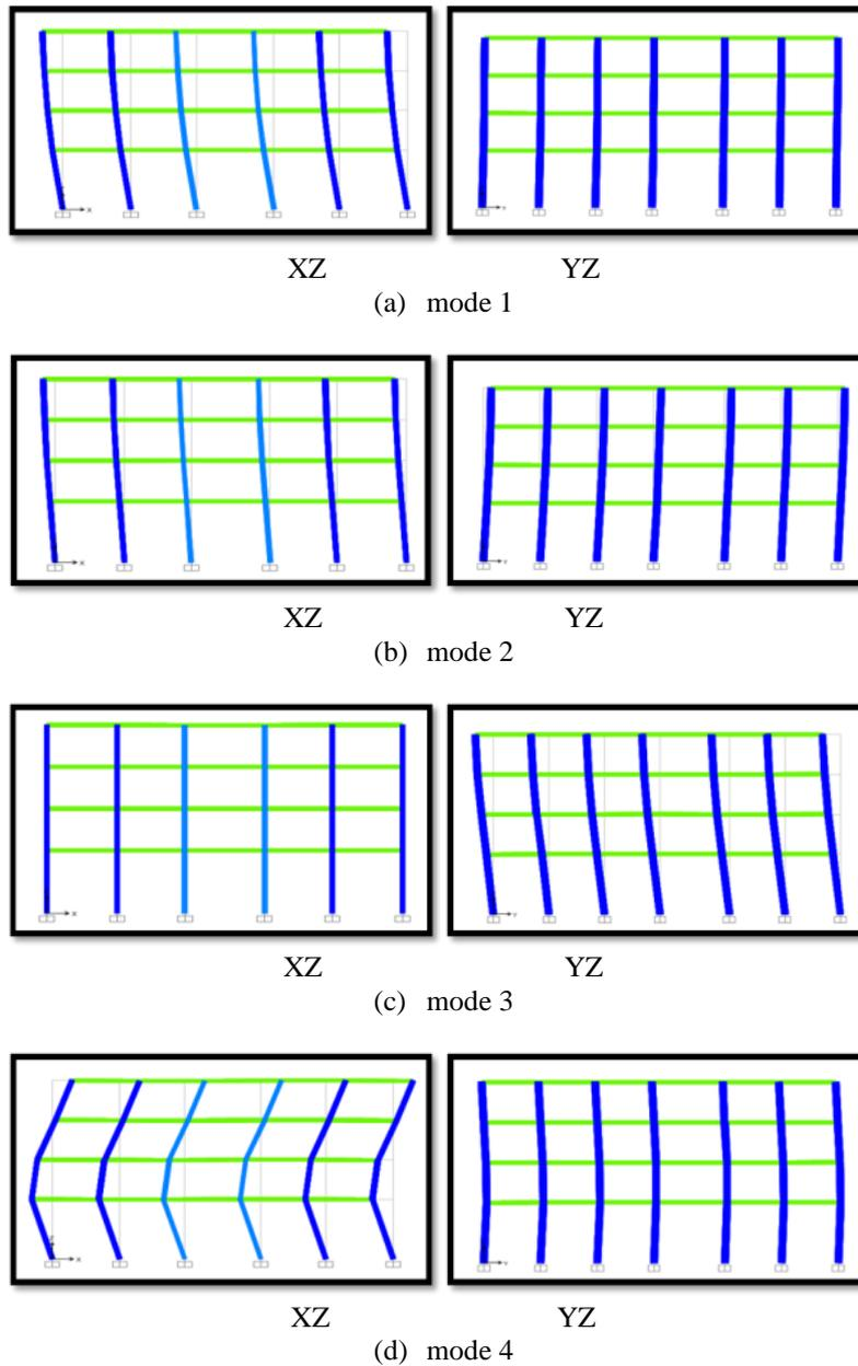
**Figure 5.** Modes Deformed Shape of building with respect to X, Y, and Z plane
