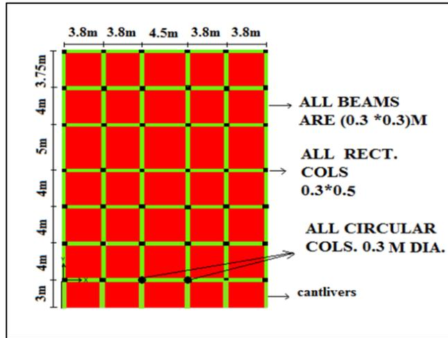
Figure 1. Typical Plan of Case Model Structure
